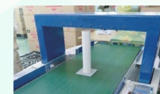
Verifying the operation of needle detectors
